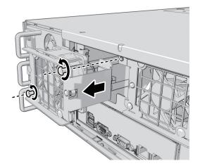
Figure 2. Replacing a CPU Fan
